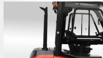
Tubo de escape vertical
